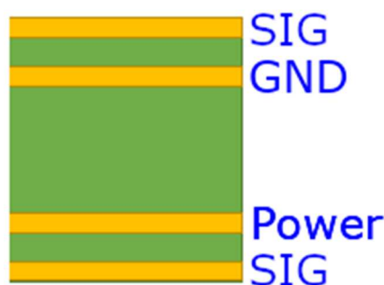
Figure 7: The classic SIG – GND – Power – SIG stack-up.
